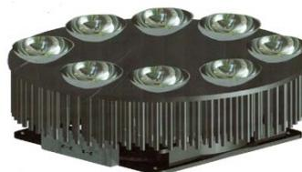
Figure 1 shows the basic unit—a silent-fan, active-cooled pin-fin heat-sink weighing less than 1.6Kg--- can accommodate over 400 watts of LED power (eight 50-watt COBs).
