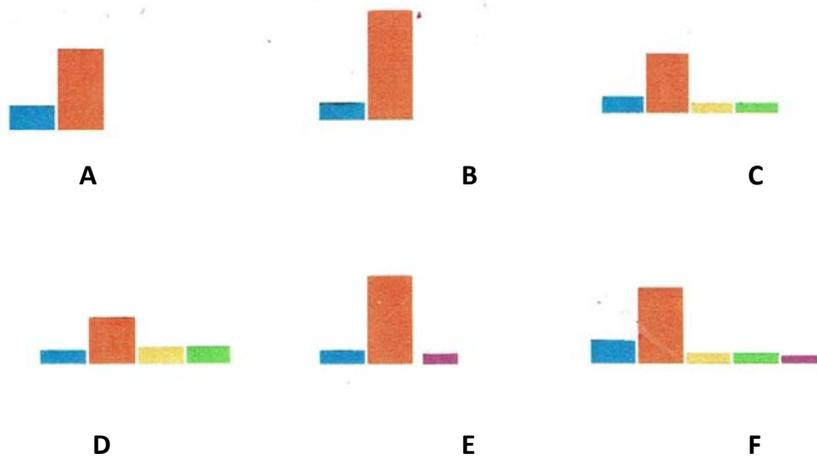
Figure 3 shows examples what is achievable just by using different combinations of five TYF COB types .The bar height shows the relative PPF energy for each wavelength color band.
